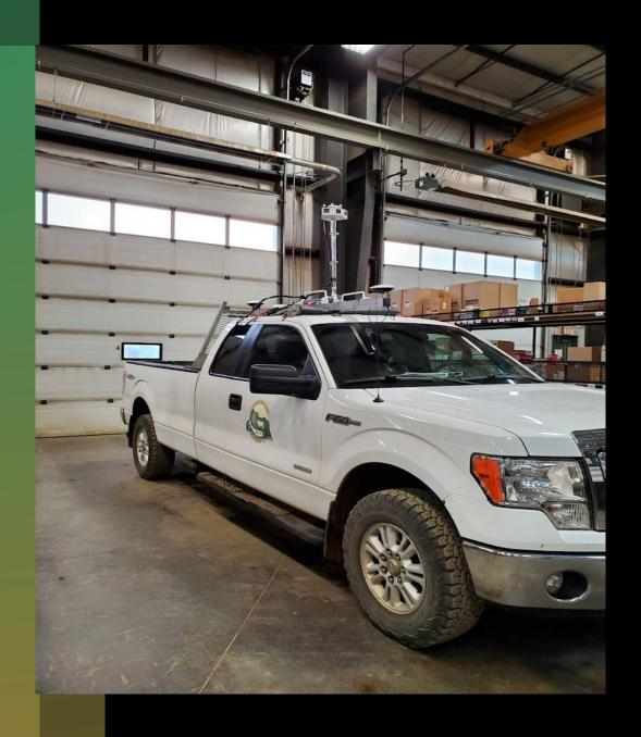
With the solid-state LiDAR and three units each data collection crew could travel at 35-40 kph to retrieve very accurate data.
