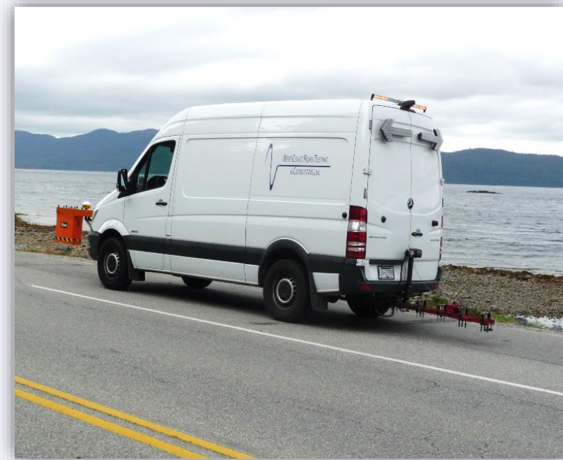
West Coast Road Testing - van mounted Falling Weight Deflectometer (FWD)
