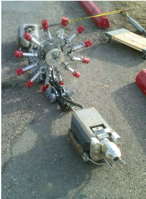
Feeder mains Concrete pipe inspections
